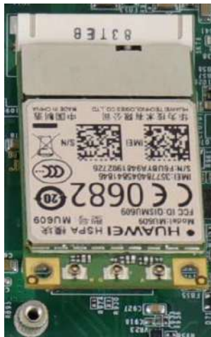
Insert on 45 degree angle Secure the module
