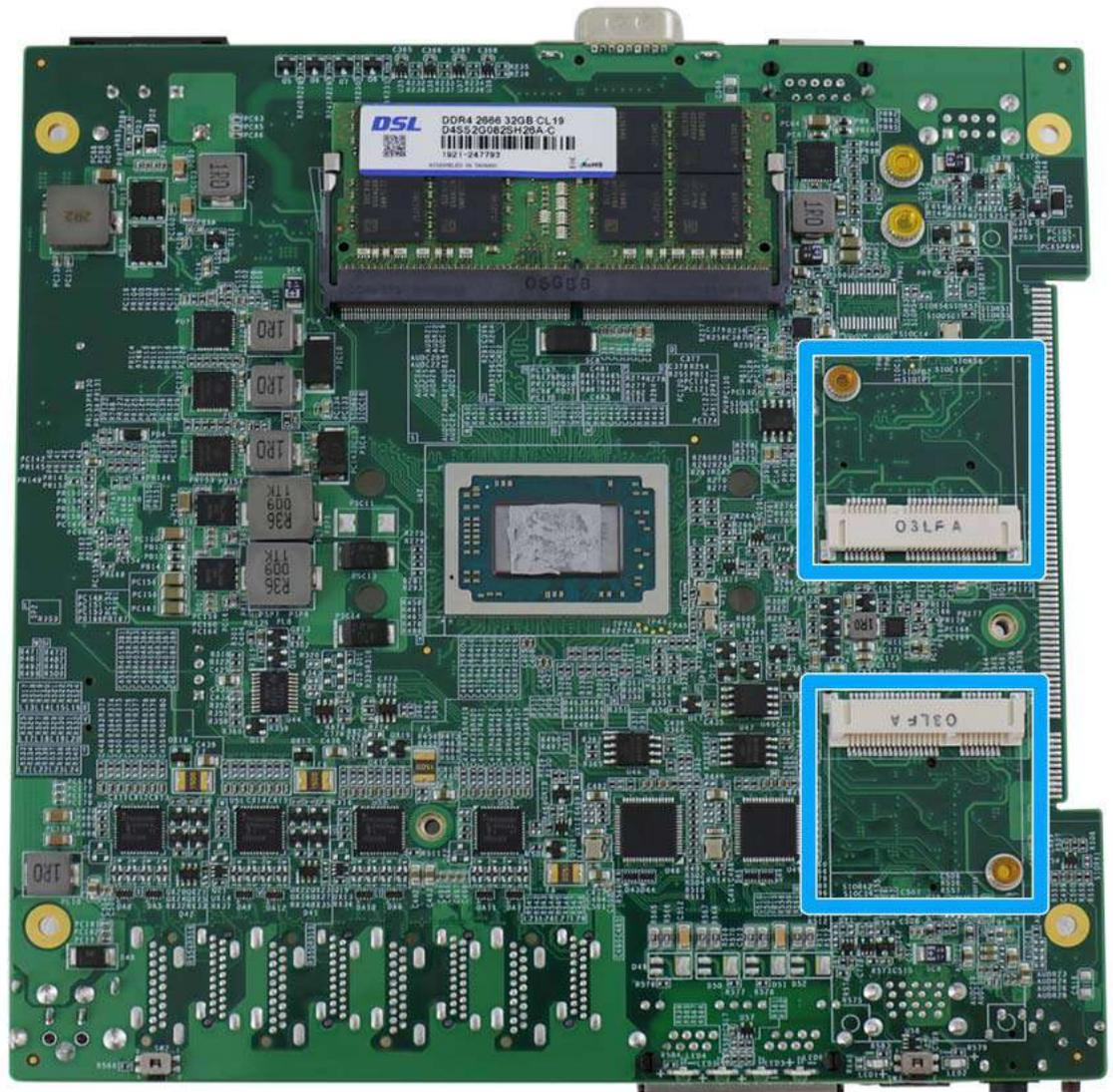
The dual half-size mini-PCIe sockets are for installing Google Edge Tensor Processing Unit (TPU). They are ideal for machine learning applications or large complex neural network models that can take up to weeks to compute but requiring only a few hours on Google TPUs.
