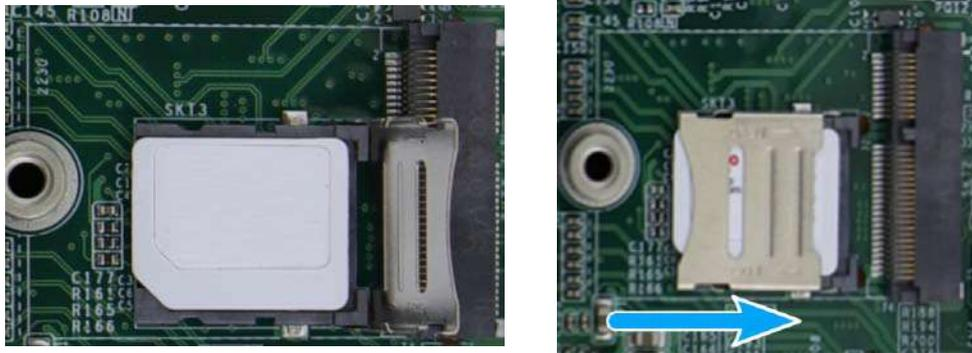
**Place into socket with orientation shown    Slide cover to secure the micro-SIM**
