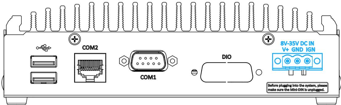
To have ignition power control for in-vehicle usage, you need to supply IGN signal to the system. The IGN input is located on the 3-pin pluggable terminal block (shared with DC power input). Below is the typical wiring configuration for in-vehicle applications.
