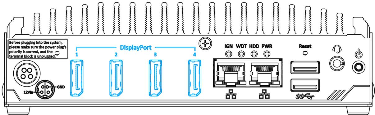
The system has four DisplayPort (DP) outputs which are digital display interfaces that mainly connect video source and carry audio to a display device. When connecting a DP, it can deliver up to 4K UHD (4096 x 2304) in resolution. The system is designed to support passive DP adapter/ cable. You can connect to other display devices using DP-to-HDMI cable or DP-to-DVI cable.
