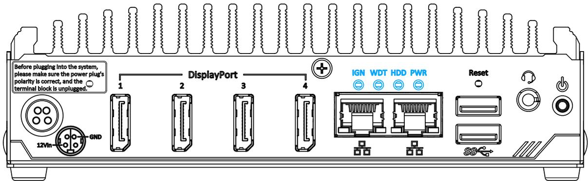
There are four LED indicators on the I/O panel: PWR, WDT, HDD and IGN. The descriptions of these LEDs are listed in the following table.
