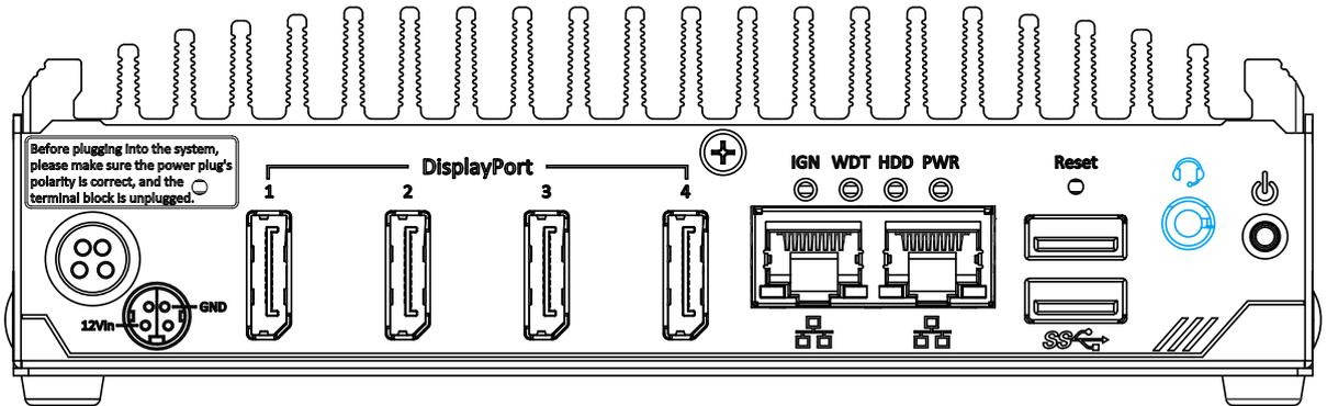
There is a female 4-pole
