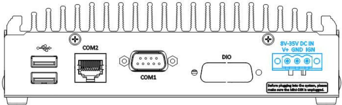
The system accepts a wide range of DC power input from 8 to 35V via a 3-pin pluggable terminal block, which is fit for field usage where DC power is usually provided. The screw clamping mechanism on the terminal block offers connection reliability when wiring DC power.
