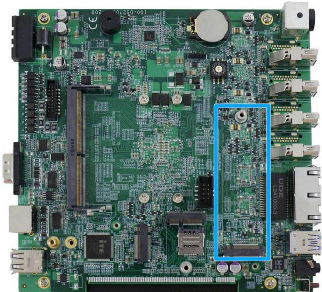
The system has an M.2 2280 slot (SATA signal only) for you to install an M.2 SATA SSD for faster access over traditional hard disk drives.
