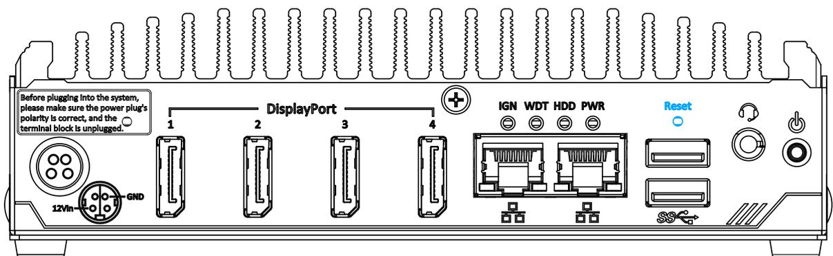
The reset button can be used to manually reset the system in case of abnormal condition. To avoid unexpected operation, the reset button is hidden behind the front panel. You need to use a pin-like object to push the reset button.
