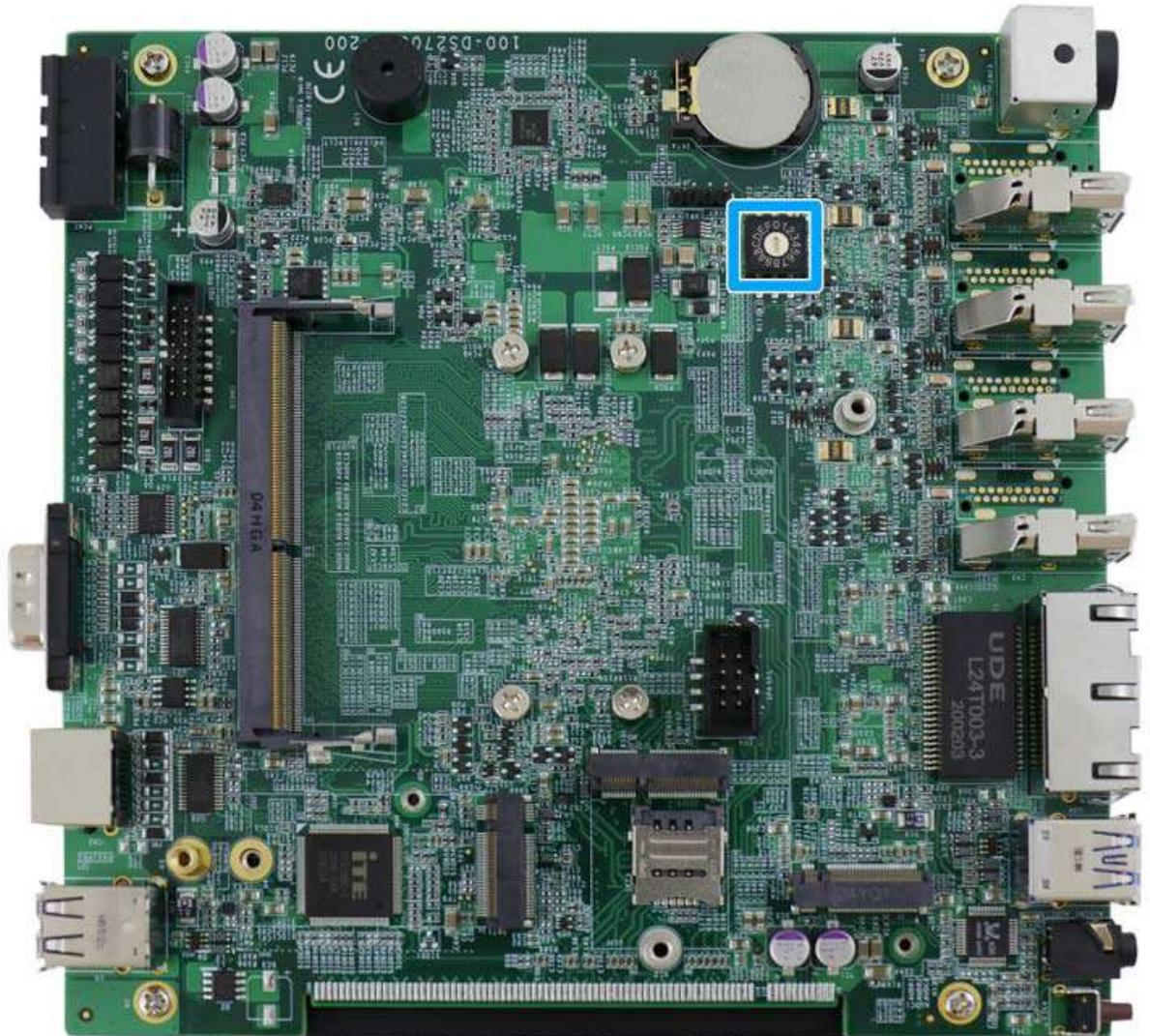
The system features an ignition control switch that has multiple modes for pre and post ignition settings. Please refer to the section [Ignition Power Control](#) for details.
