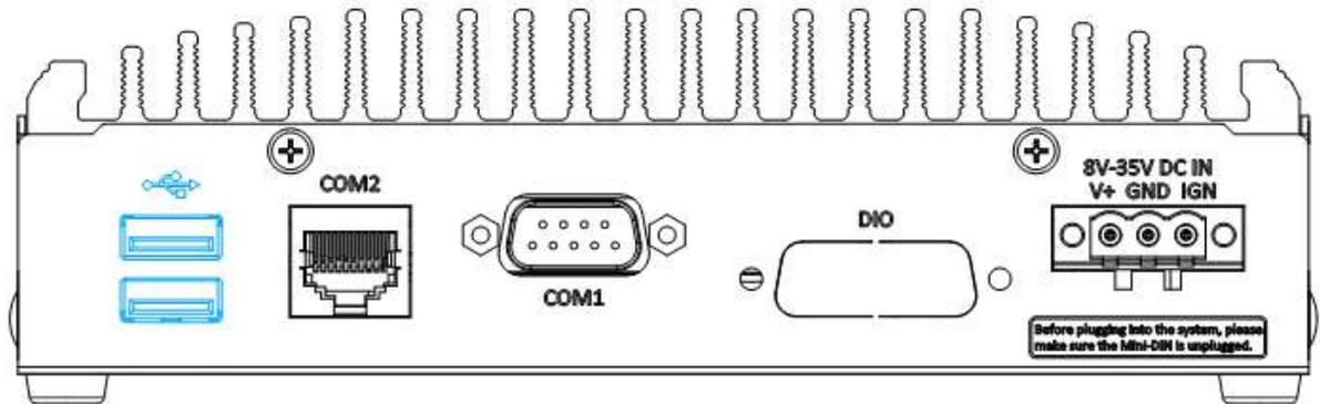
The system has two USB 2.0 ports. They are implemented by native xHCI (eXtensible Host Controller Interface) controller in H310 chipset and are compatible with USB 2.0, USB 1.1 and USB 1.0 devices. Legacy USB support is also provided so you can use USB keyboard/mouse in DOS environment.
