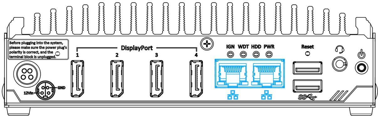
The system offers two GbE ports implemented with Intel® I210-IT controllers. Each port has one dedicated PCI Express link for maximum performance. When an Ethernet connection is established, the LED indicators on the RJ45 connector represents the following connection statuses:
