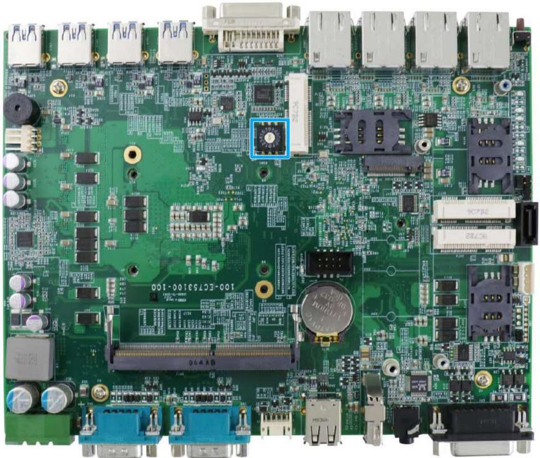
The ignition power control switch features multiple modes for pre and post ignition settings. Please refer to the section [Ignition Power Control](#) for details.
