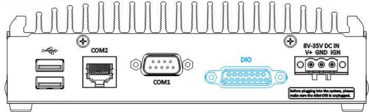
With the cable Cbl-IDC216F-DB15M-4.5CM” connected onto the motherboard, and female DB15 connector installed onto the panel, the digital input (DI) and digital output (DO) function provides four digital input and four digital output on the rear panel of the system.
