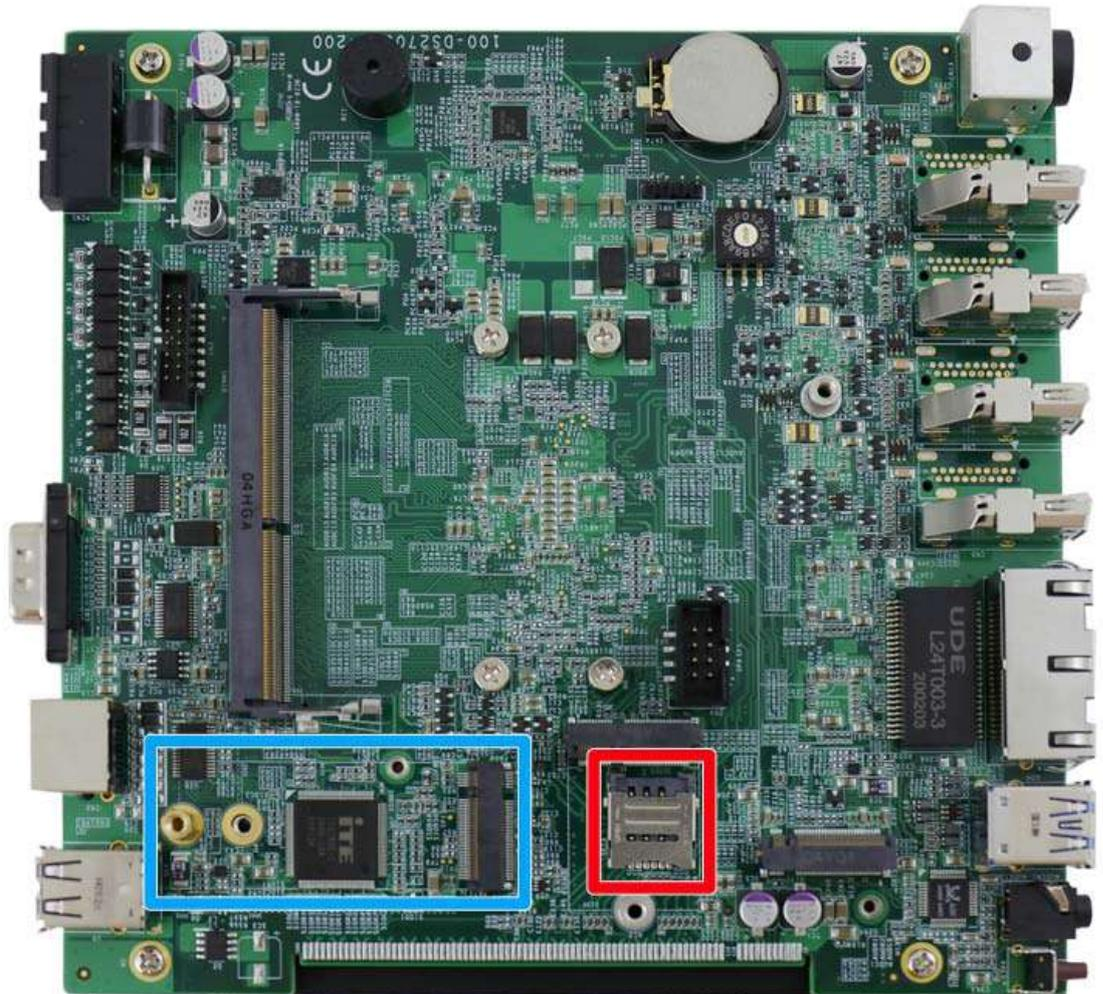
The system has one M.2 3042/ 3052 B key socket (in **blue**) with USB3.1 Gen 1 and USB 2.0 signal for 4G/ 5G module installation. There is also a corresponding micro-SIM SIM card slot (in **red**).
