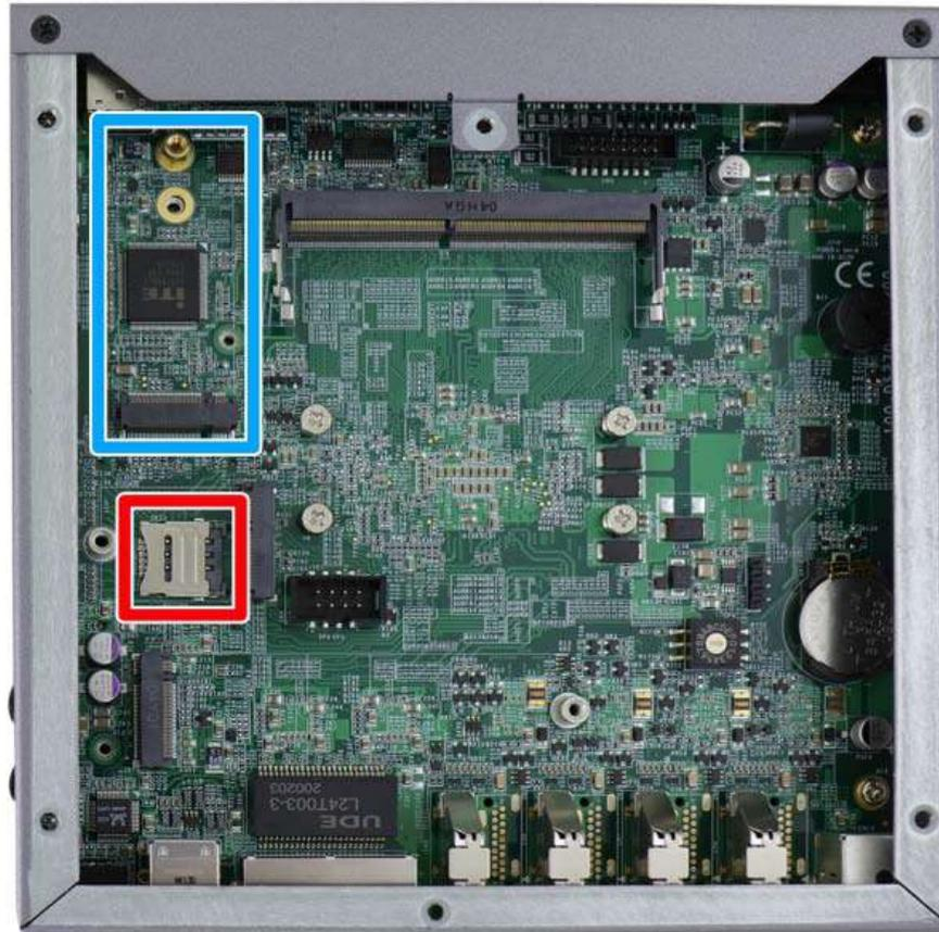
1. To install the micro-SIM SIM card, slide the metallic cover in the direction shown and lift it to expose the socket and gold fingers.
