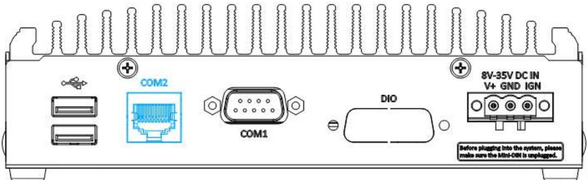
COM 2 port is a RS-232 port that uses an RJ 50 connection. The RJ 50 connection is designed to be compatible with existing digital signage players.
