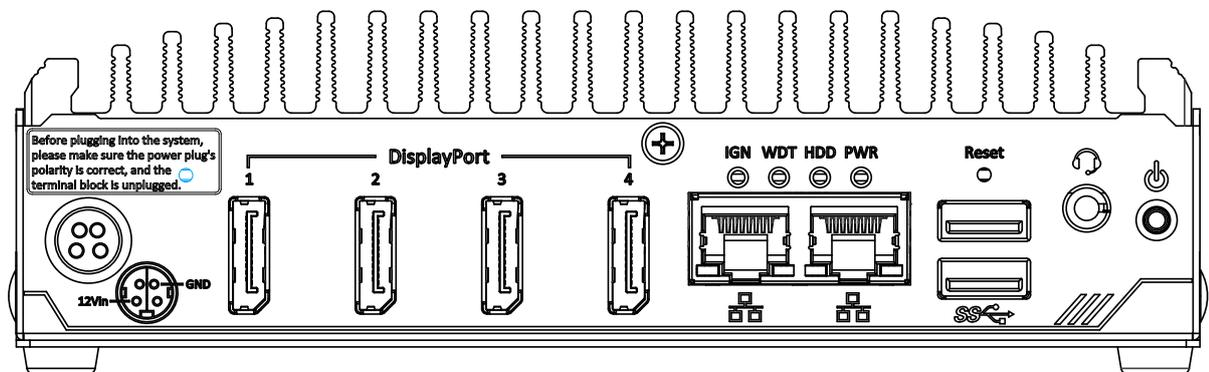
The CMOS Reset button is used to manually reset the motherboard BIOS in case of system halt or malfunction. To avoid unexpected operation, it is purposely placed behind the panel. To reset, please use the tip of a pen, press and hold for at least 5 seconds to reset the BIOS.
