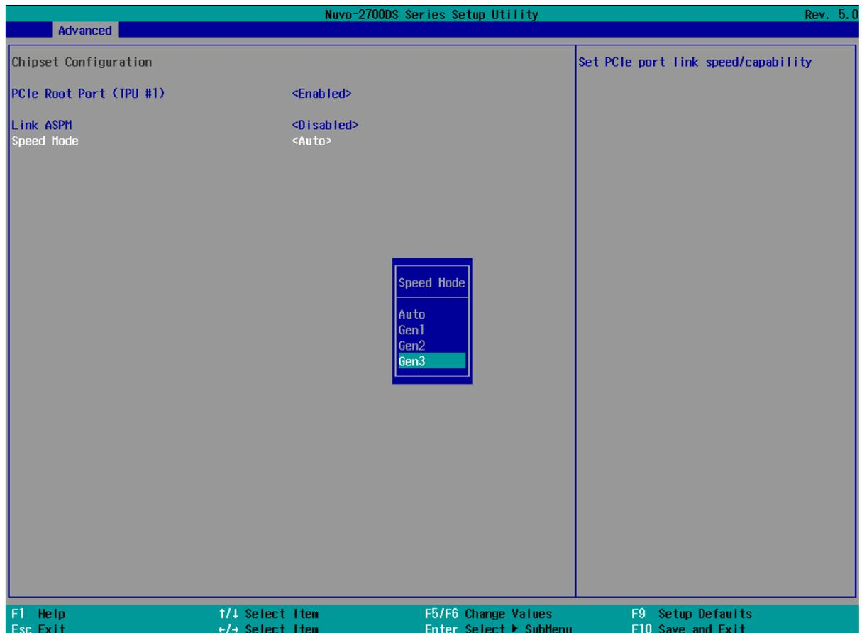
To configure PCIe Root Port (TPU):
