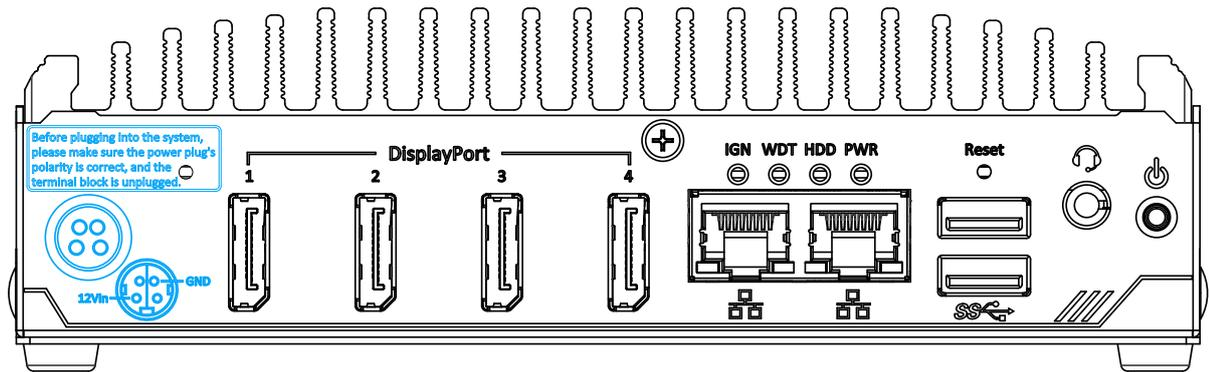
The system accepts a DC power input of 12V. DO NOT plug in the 12V DC connector and the 3-pin terminal connector. The system only requires one or the other for operation.
