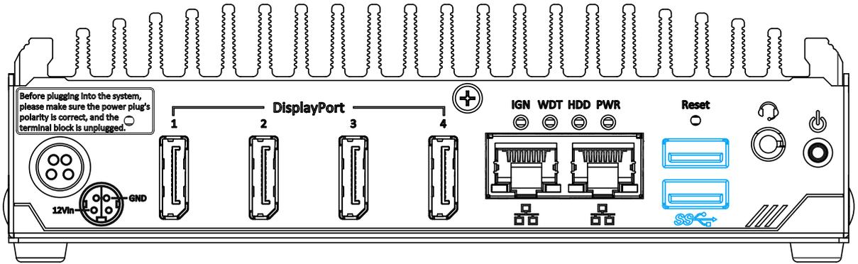
The system offers two USB 3.1 Gen1 (SuperSpeed USB) ports on its front panel with screw-lock mechanism. They are backward-compatible with USB 2.0, USB 1.1 and USB 1.0 devices. Legacy USB support is also provided so you can use USB keyboard/mouse in DOS environment while USB 3.1 Gen1 driver is supported natively in Windows 10.
