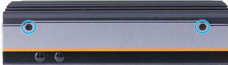
**Right side chassis screws securing the heatsink**
