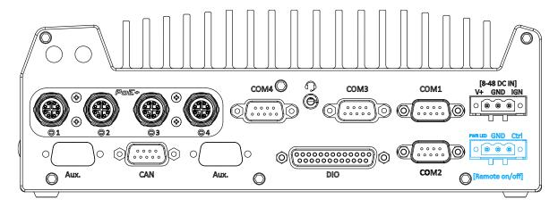
The "Remote On/ Off" 3-pin connection allows for external switch extension. It is useful when the system is placed in a cabinet or a not easily accessed location. You may connect an external status LED (20mA) indicator by connecting to PWR LED and GND.
