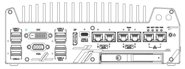
The CMOS Reset button is used to manually reset the motherboard BIOS in case of system halt or malfunction. To avoid unexpected operation, it is purposely placed behind the panel. To reset, disconnect the DC power input, and use the tip of a pen to press and hold for at least 5 seconds to reset the BIOS.
