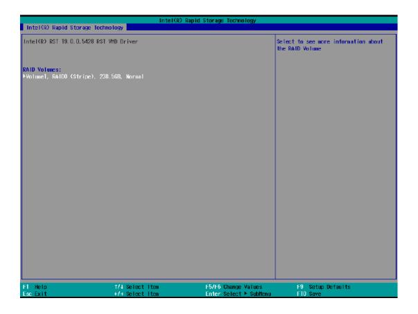
10. Press F10 to save and Esc to exit the Intel® Rapid Storage Technology configuration page.
