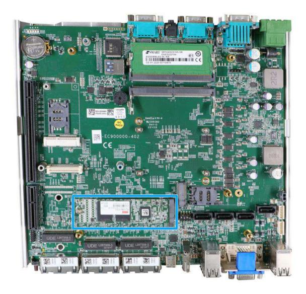
The system has a Gen4 x4 PCIe M.2 2280 slot for you to install an NVMe SSD. The M.2 NVMe SSD offers significantly better system performances when compared to a 2.5" SSD.
