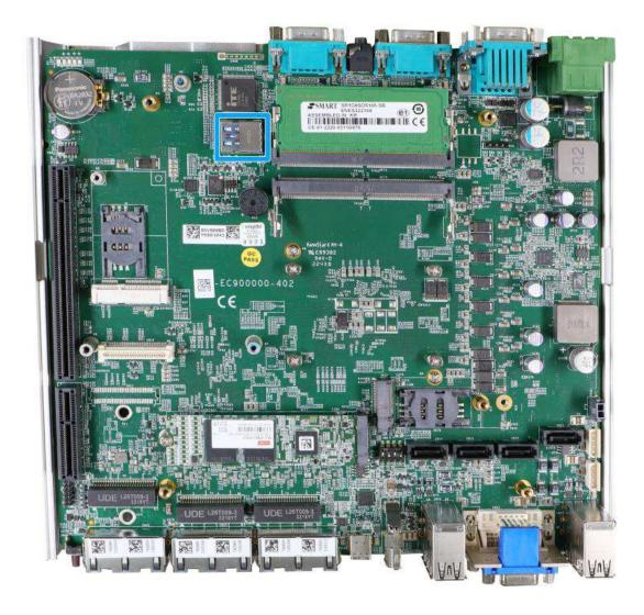
The system's motherboard has an internal USB2.0 port on the PCBA. You can utilize this USB port to connect a USB protection dongle inside the chassis of the system.
