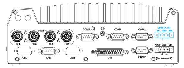
To have ignition power control for in-vehicle usage, you need to supply IGN signal to the system.
