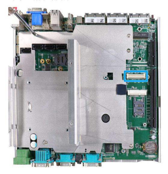
MezIO<sup>TM</sup> is an innovative interface designed for integrating application-oriented I/O functions into an embedded system. It offers computer signals, power rails and control signals via a high-speed connector. MezIO<sup>TM</sup> is also mechanically reliable benefited from its 3-point mounted mezzanine structure. A MezIO<sup>TM</sup> module can leverage these signals to implement comprehensive I/O functions.
