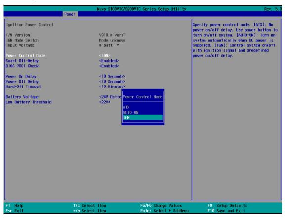
4. If you wish to set the power on delay time from when you start-up the vehicle, highlight and select "Power On Delay", select the timing according to your needs and press Enter.
