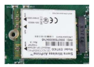
5. Gently press down and secure the module with an M3 P-head screw.
