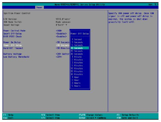
6. If you wish to set the a hard power off timing, select "Hard-Off Timeout", select the timing according to your needs and press Enter.
