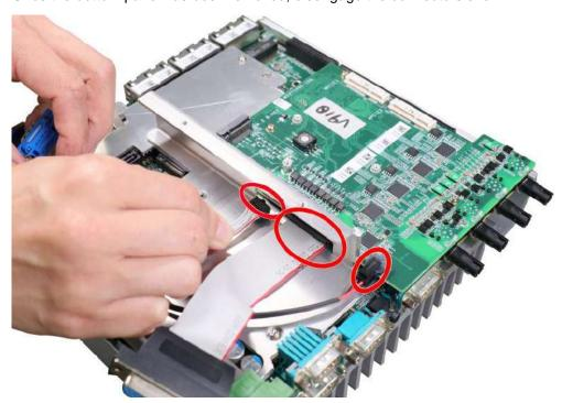
9. Remove the MezIO<sup>TM</sup> module by unscrewing the screws shown and gently lift to separate it from the motherboard.
