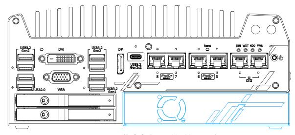
Neousys' patented expansion Cassette (R.O.C. Patent No. M456527) provides a separated compartment to accommodate an add-on card. It effectively manages thermal conditions of both the system and the add-on card. The modular concept brought by Cassette module also reduces the complexity of installing and replacing an add-on card in the fanless controller.
