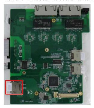
4. Insert the module on a 45 degree angle.
