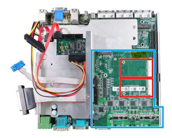
There are two additional full-size mini-PCIe sockets (indicated in **red**) available on the MezIO<sup>™</sup> module (indicated in **blue**). They are implemented with USB signals only have better compatibility with off-the-shelf 3G/ 4G mini-PCIe modules. For customers who want to install 3G/ 4G module(s), please take advantage of these two mini-PCIe sockets and the associated SIM slots.
