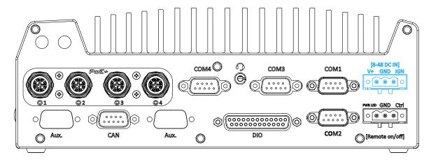
The system accepts a wide range of DC power input from 8 to 48V via a 3-pin pluggable terminal block, which is fit for field usage where DC power is usually provided. The screw clamping mechanism on the terminal block offers connection reliability when wiring DC power.
