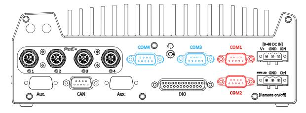
The system provides four COM ports for communicating with external devices. These COM ports are implemented using industrial-grade ITE8786 Super IO chip (-40 to 85°C) and provide up to 115200 bps baud rate.
