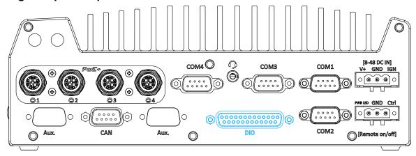
The system provides 4x isolated digital input channels and 4x isolated digital output channels. The DIO functions support polling mode I/O access and DI change-of-state interrupt. Please refer to digital I/O pin definition on the following page and <u>Watchdog Timer & Isolated DIO</u> for information on wiring and programming the isolated DIO channels.
