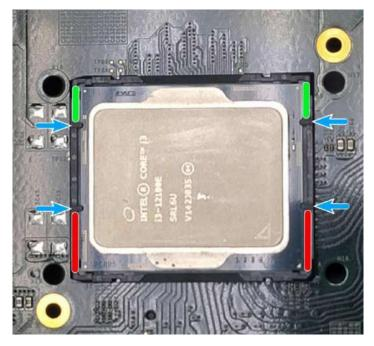
8. Make sure all thermal pad residues have been cleaned on both sides of the retention bracket. Place the CPU retention bracket (holder) on top of the CPU and hold it in place. Make sure the indicator triangle engraved on the CPU's integrated heat spreader (IHS) and the triangle indicator on the retention bracket are positioned in the same corner (indicated by blue circles).
