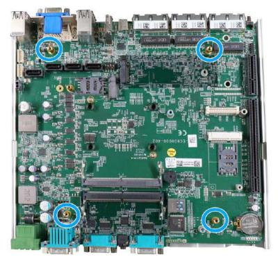
Secure motherboard with four screws
