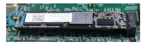
4. Please remember to remove the thermal pad protector film off the heatsink/ support frame for NVMe SSD.
