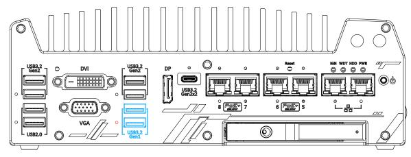
The system's USB 3.2 Gen1x1 ports (5Gbps) are implemented via native xHCI (eXtensible Host Controller Interface) controller and are backward compatible with USB 2.0, USB 1.1 and USB 1.0 devices. UEFI USB is also supported so you can use USB keyboard/mouse in UEFI shell environment. Indicated in **red** is a screw-lock hole for the corresponding USB port. xHCI driver is supported natively in Windows 10, therefore you do not need to install the xHCI driver prior to utilizing USB functions.
