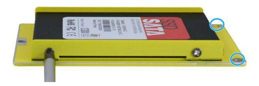
At the tray opening, you should be able to locate the 22-pin SATA cable, connect it to the installed HDD/ SSD.
