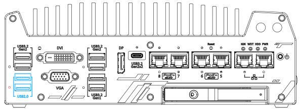
The USB2.0 ports are implemented via native xHCI (eXtensible Host Controller Interface) and are backward compatible with USB 1.1 and USB 1.0 devices. UEFI USB support is also provided so you can use USB keyboard/ mouse in UEFI shell environment. Indicated in **red** is a screw-lock hole for the corresponding USB port.
