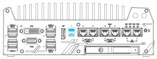
The system's USB 3.2 Gen2x2 type-C port offers up to 20Gbps of data transfer bandwidth, and is implemented via the native xHCI (eXtensible Host Controller Interface) controller. Indicated in **red** is a screw-lock hole for the corresponding USB port.
