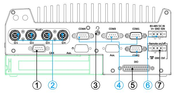
The rear panel features four RJ45 or M12 PoE ports, CAN bus, digital I/O, four COM ports, ignition control switch, 3-pin terminal and remote 3-pin on/ off control.
