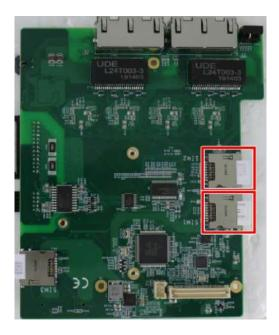
Micro SIM slots are inserted underneath the mini-PCle slots on  $MezIO^{TM}$  module
