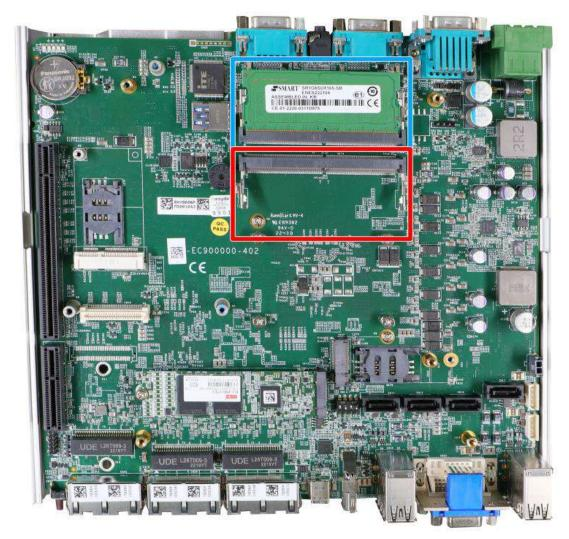
The system motherboard supports two DDR5 4800 SODIMMs memory module up to 64GB. Each slot supports single module SODIMM up to 32GB capacity. If you are installing a memory module, please install into the slot indicated in blue. When both slots are occupied, it is recommended that the operating ambient temperature does not exceed 60°C to avoid thermal throttling.
