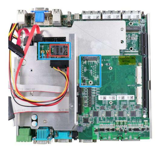
M.2 slot on MezlO<sup>™</sup> module and on the motherboard (accessible without removing heatsink/ support frame)
