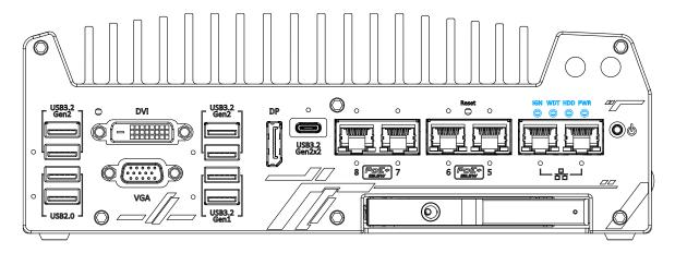
There are four LED indicators on the I/O panel: IGN, WDT, HDD and PWR. The descriptions of these four LED are listed in the following table.
