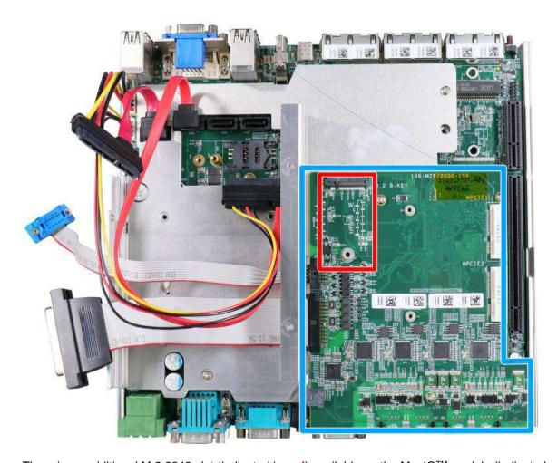
There is an additional M.2 2242 slot (indicated in **red**) available on the MezlO<sup>™</sup> module (indicated in **blue**). To expand wireless networking capability, users can install off-the-shelf 4G/3G modules and access the internet via the provider's network.
