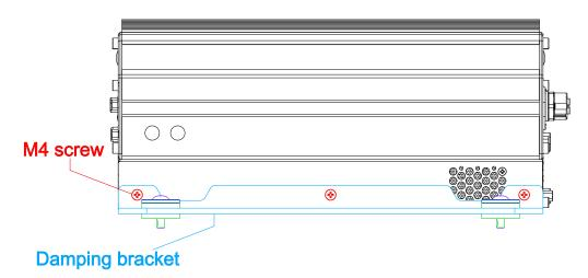
Place the system on a flat surface, insert the sleeves into the anti-vibration grommets and secure it with M4 screws.
