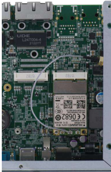
Clip on the IPEX-to-SMA cable
