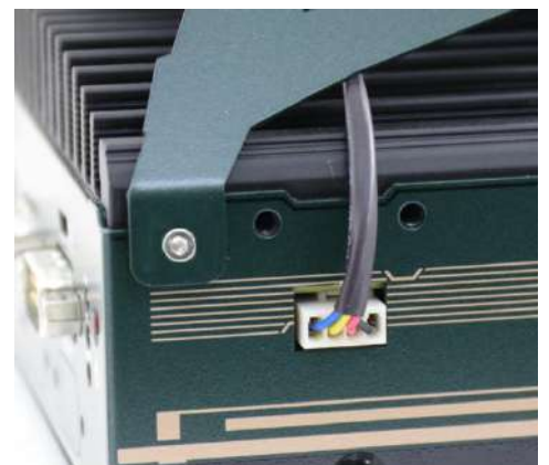
Plug in the 4-pin power connector
