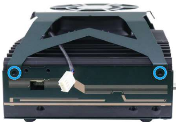
Secure the two screws
