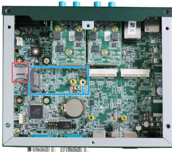
M.2 B key and internal SIM card slot
