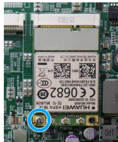
Secure the card with a screw
