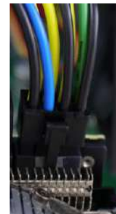
6-pin power connector on graphics card
