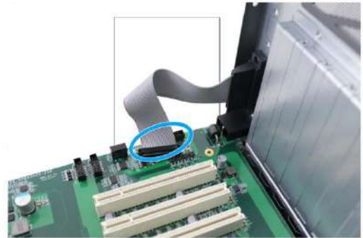
Disconnect DIO connector
