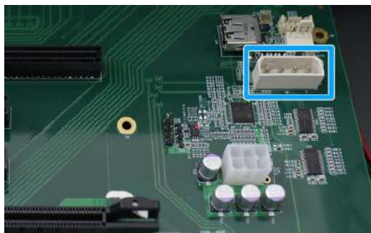
4-pin molex connector for PoE card
