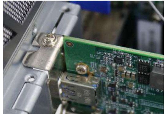
Secure bezel with screw
