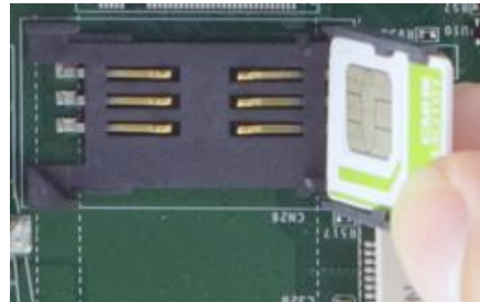
Insert SIM card with pins facing up
