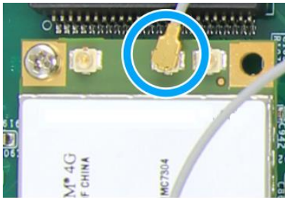
Clip on IPEX-to-SMA cable
