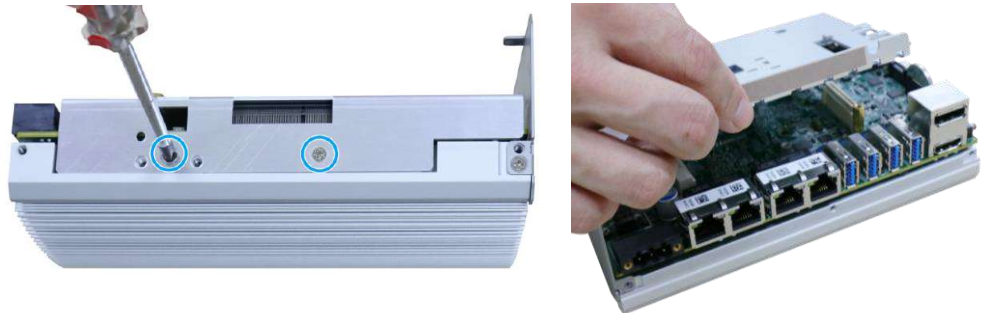
Remove screws securing heat spreader
