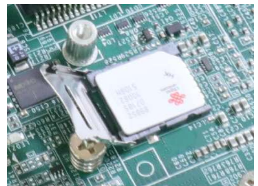
Flip open the holder and place SIM
