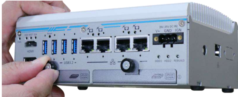
Turn thumb screw anti-clockwise
