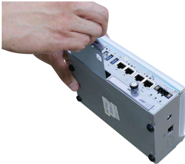
Retrieve tray out of I/O panel
