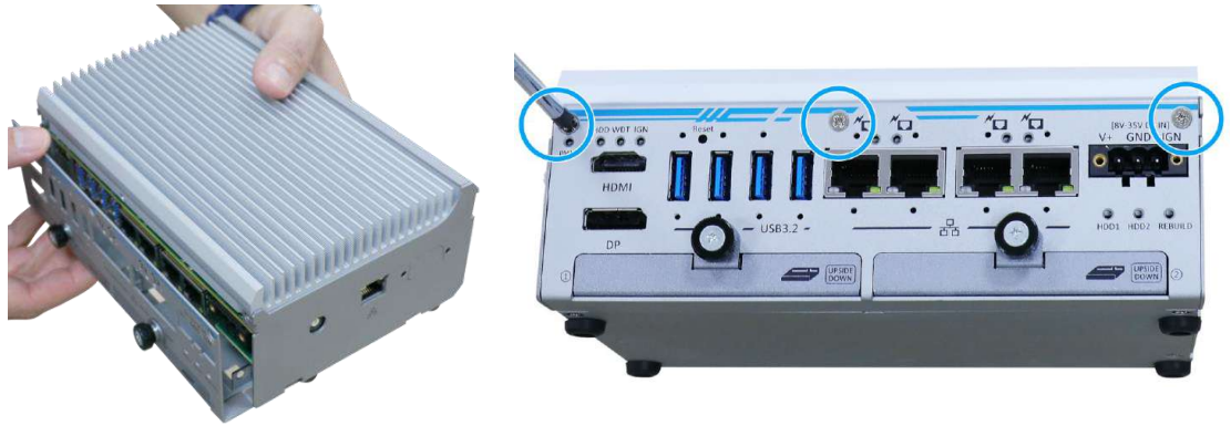
Install front panel
