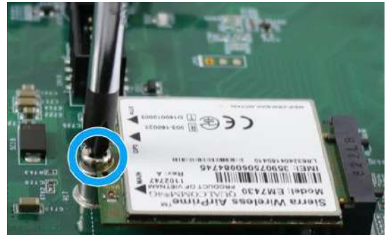
Secure the module with a screw
