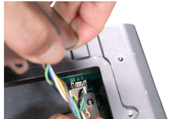
Connect from the motherboard side
