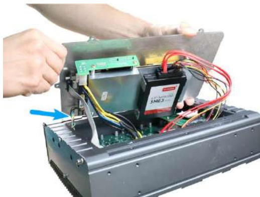
Connect the 4-pin power connector
