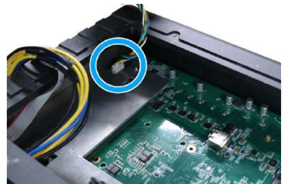
Unplug the 4-pin ATX connector
