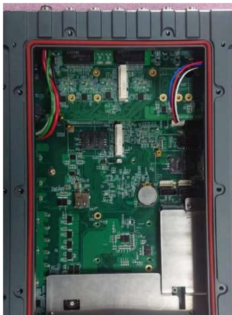
O-ring seated properly in the groove
