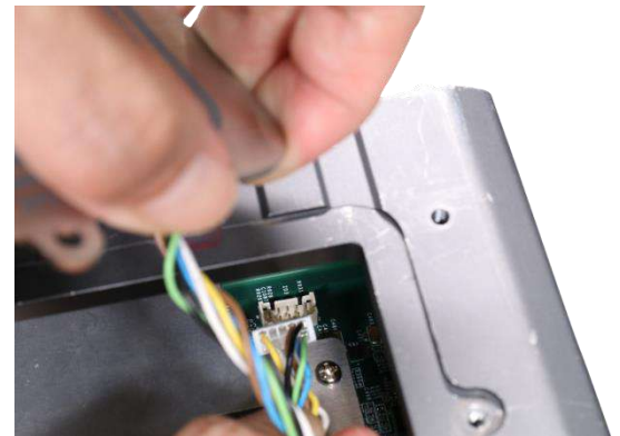
Connect from the motherboard side
