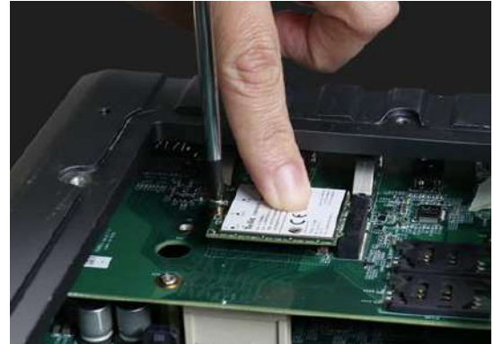
Secure the module with a screw
