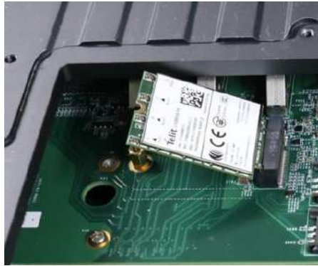
Insert into slot on a 45 degree angle
