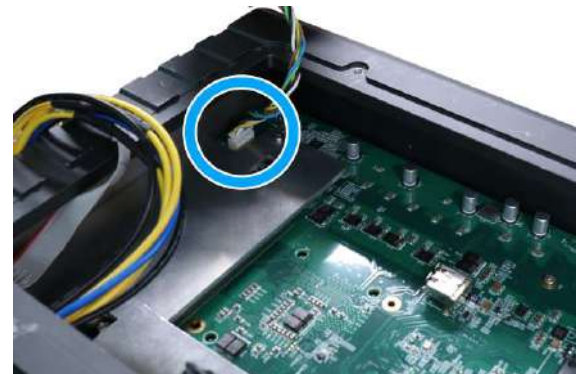
Unplug the 4-pin ATX connector
