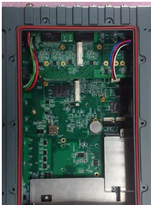
O-ring seated properly in the groove
