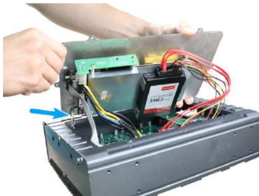
Connect the 4-pin power connector
