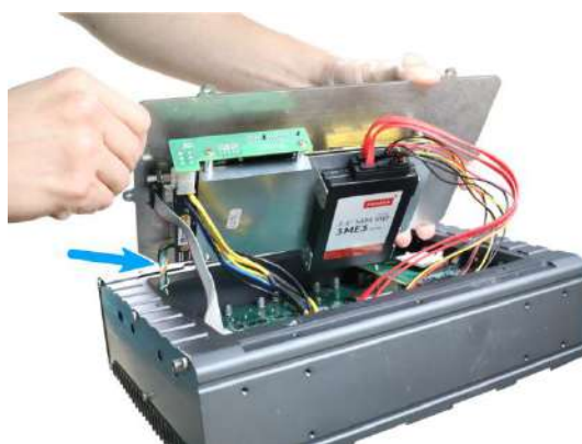
Unplug the DB9 connection to the PB unit
