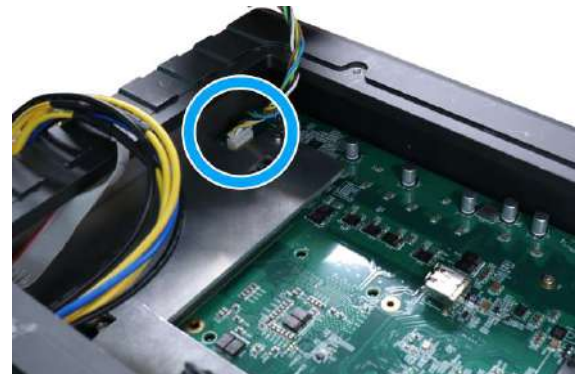
Unplug the 4-pin ATX connector
