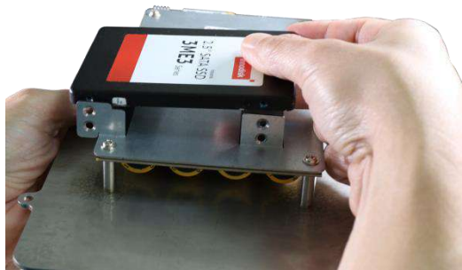
Place hard drive in between brackets
