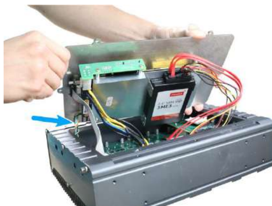
Disconnect the 4-pin power connector
