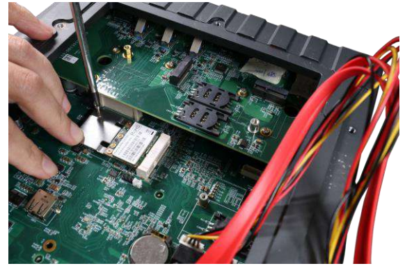
Secure the module with a screw
