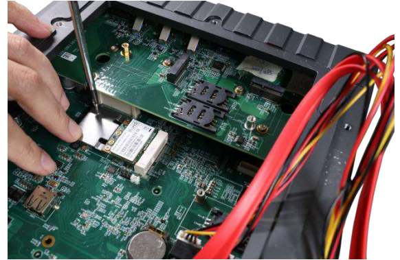
Secure the module with a screw
