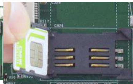
Insert SIM card with pins facing up
