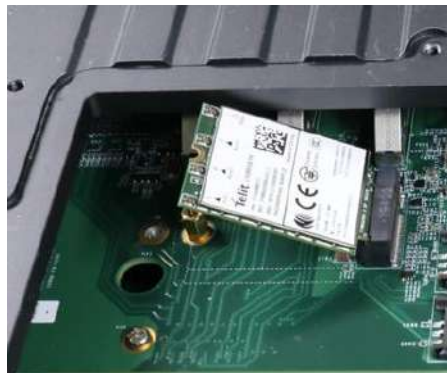
Insert into slot on a 45 degree angle
