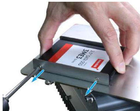
Remove the two screws on each side of the hard drive
