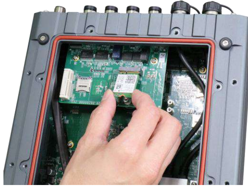
Insert on a 45 degree angle
