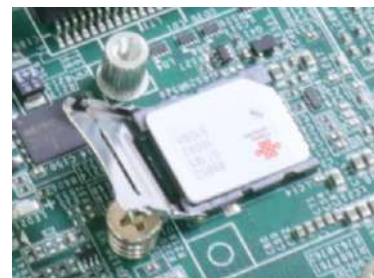
Flip-open the holder and place SIM
